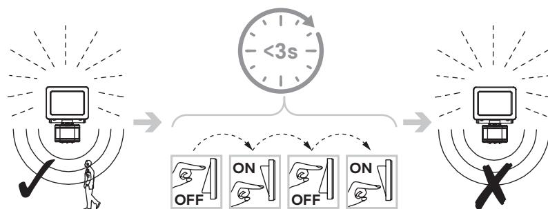
**EN** Deactivate motion sensor and keep light on
