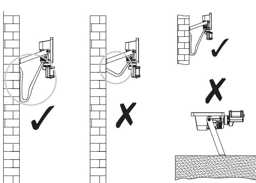
**EN** Loop the mains cable lower than the connector.
