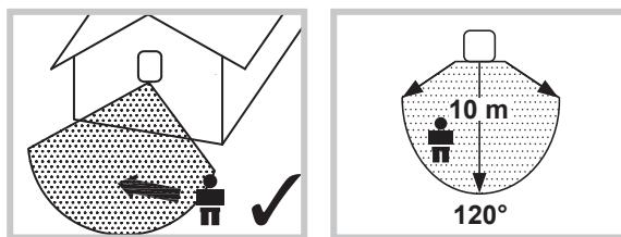
**EN** To set a desired product setting (Time, Lux sensibility or sensor range) keep rotating the corresponding knob until the lamp lights up.
