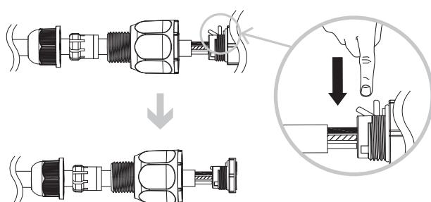
**EN** The connector is designed for ease of installation and to ensure a good electrical connection. With enough force, wires can be pulled out of the connector even when the lever is down. Once installed, the cable gland ensures a tight, durable connection (step 8).
