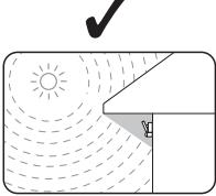
EN Avoid sunlight falling onto the lens of sensor
