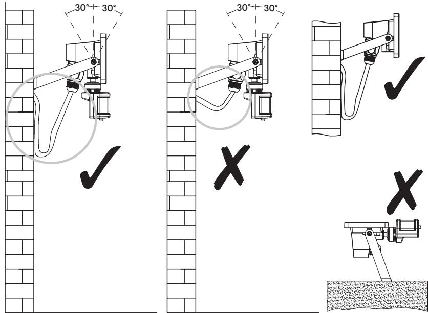
EN Loop the mains cable lower than the connector.
