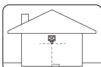
**EN** Mount the sensor perpendicular to the ground
