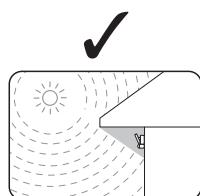
**EN** Avoid sunlight falling onto the lens of sensor
