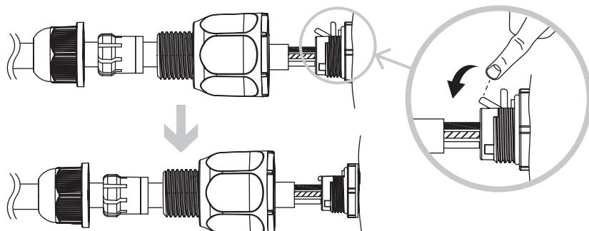
**EN** The connector is designed for ease of installation and to ensure a good electrical connection. With enough force, wires can be pulled out of the connector even when the lever is down. Once installed, the cable gland ensures a tight, durable connection (step 7).
