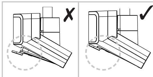
**EN CAUTION:** Cover must be closed completely for water ingress protection.
