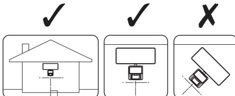
**EN** Mount the sensor perpendicular to the ground
