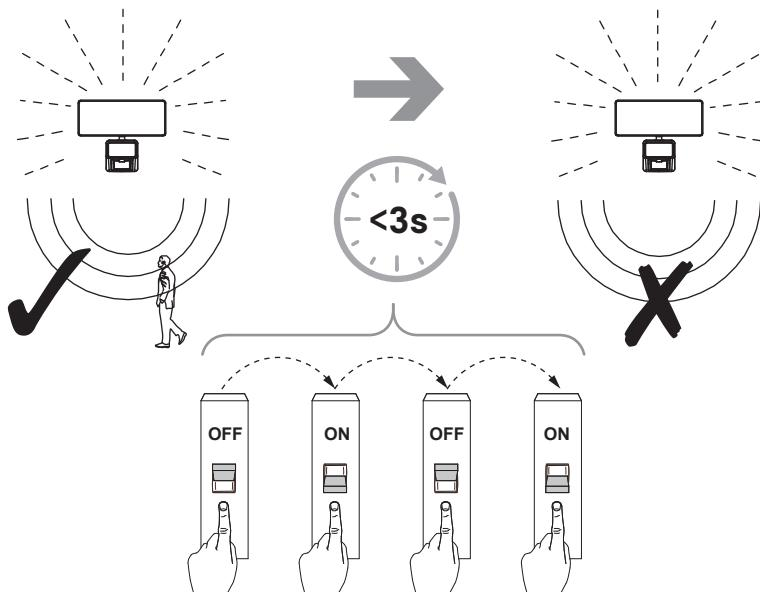
**EN** Deactivate motion sensor and keep light on
