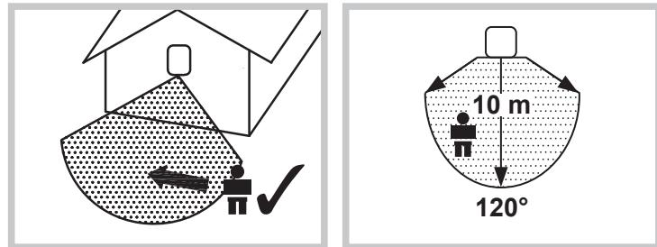
**EN** To set a desired product setting (Time, Lux sensibility or sensor range) keep adjusting the corresponding knob until the lamp lights up.
