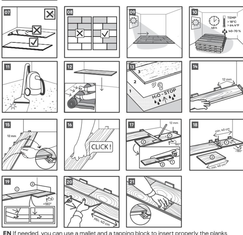
**EN** If needed, you can use a mallet and a tapping block to insert properly the planks between them as below.
